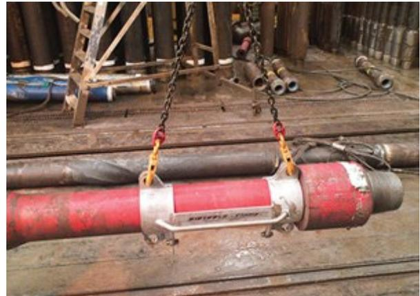
Fig. 5. RIGTOOLS' clamp tool aids sub lifting and handling.
